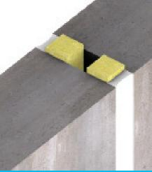
NOTE: If the fire risk is from both sides of the gap, then the sealant should be installed on both sides.
