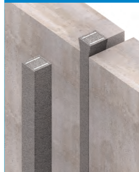
Sealing movement joints at junction for walls.
