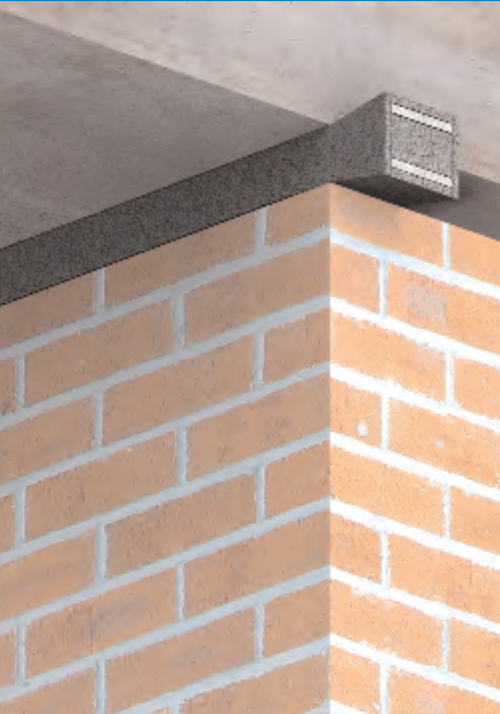
Sealing movement joints at junctions for walls and floors.
